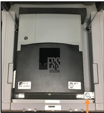
Interior Security Lock
